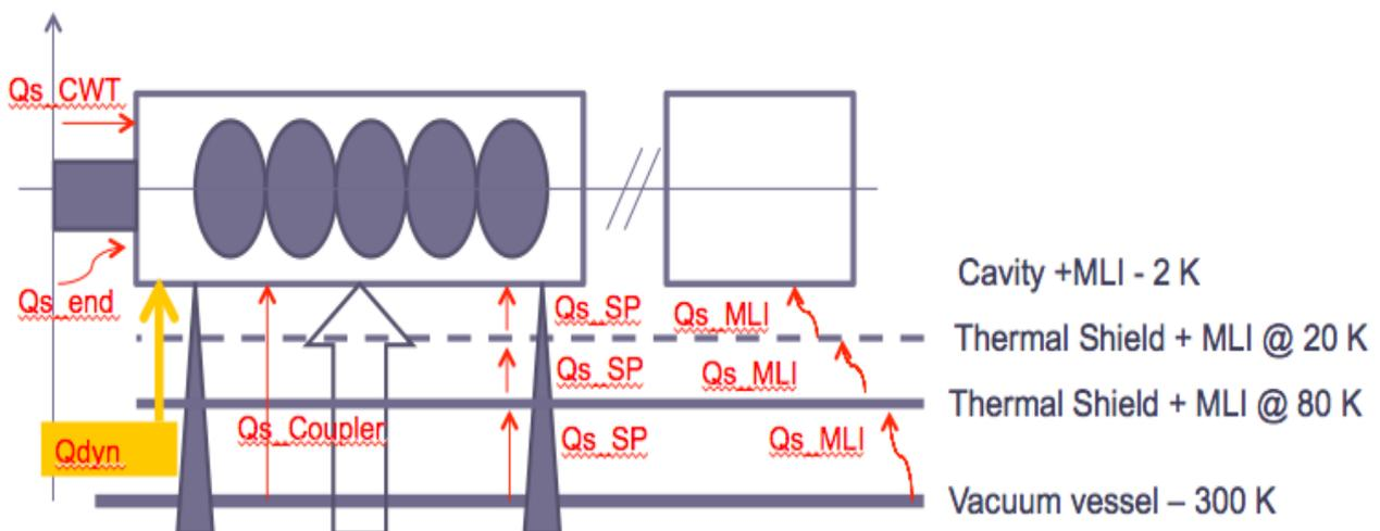
Figure 2: Main cryomodule heat transfer flow scheme of the heat transfer (HOM, tuner and instrumentation contributions are not shown)
