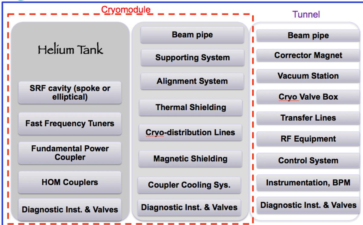
Figure 1: Cryomodule Breakdown Structure and Interfaces
