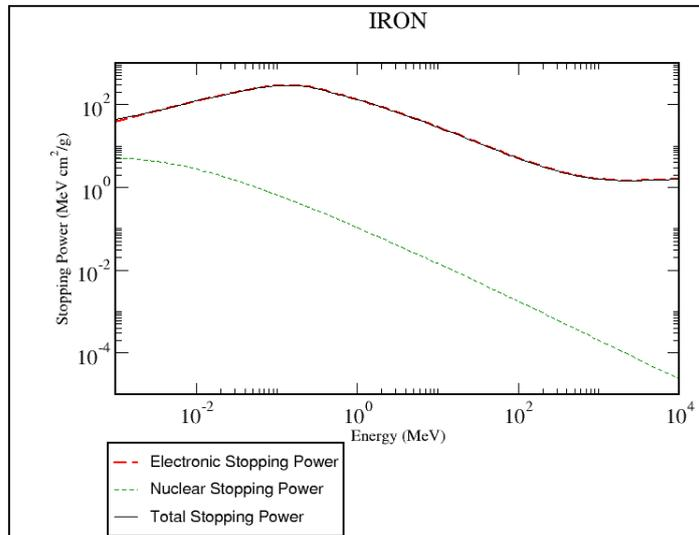
Figure 2.2: Proton stopping power in iron as a function of it's energy
