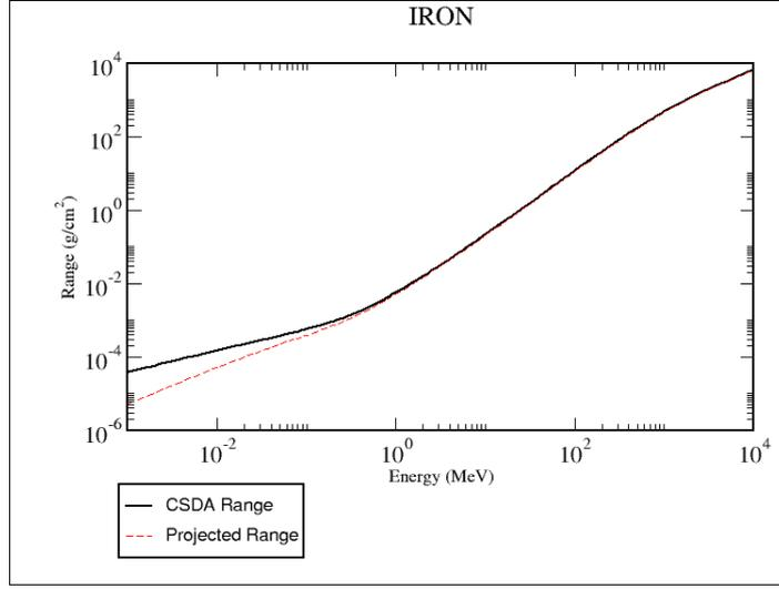
Figure 2.3: Proton range in iron as a function of it's energy
