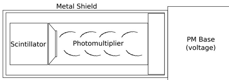
Figure 3.1: Schematic diagram of a scintillator detector.
