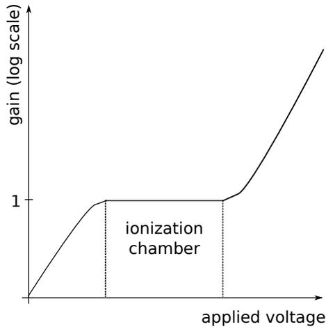
Figure 3.3: Different regions of operation of gas-filled detector.
