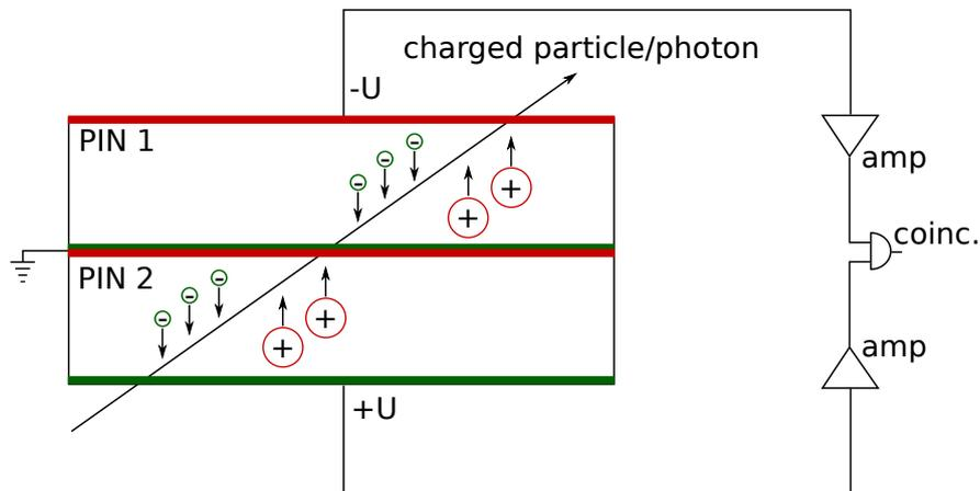
Figure 3.5: Scheme of two PIN diodes driven in coincidence.
