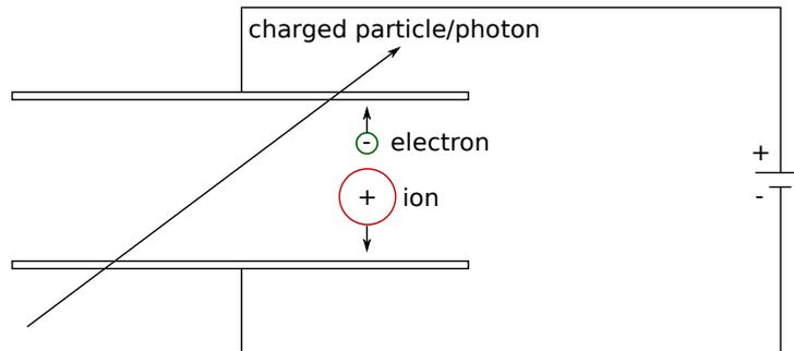
Figure 3.2: Ionization chamber working mechanism.
