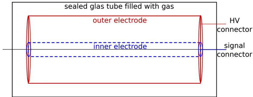
Figure 3.4: Ionization chamber working mechanism.
