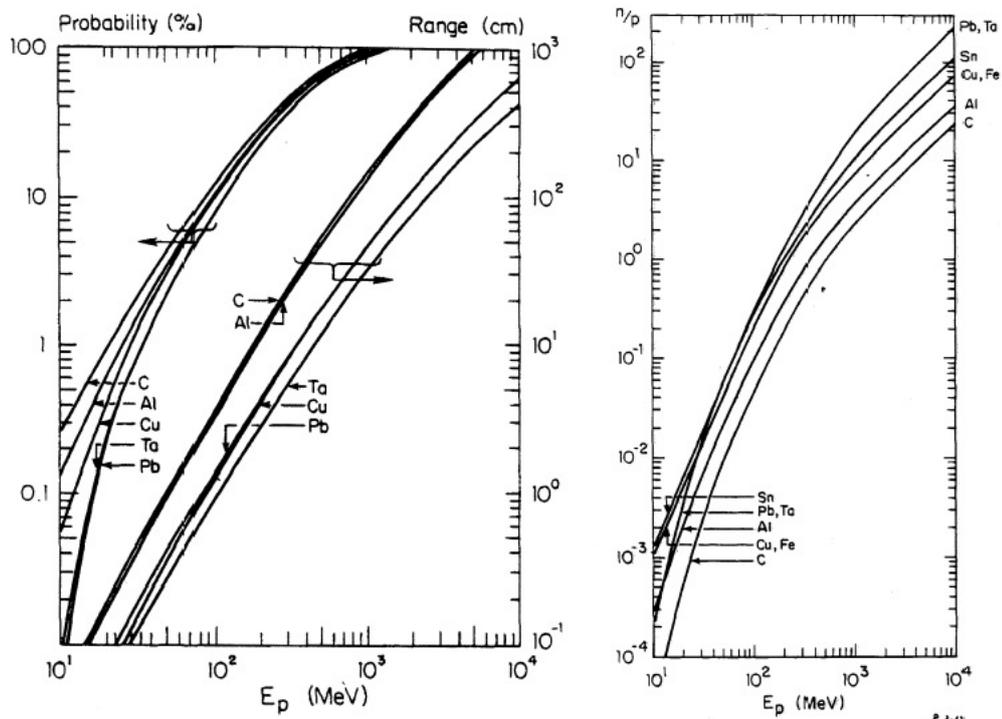
Figure 2.4: Left: probability of proton inelastic nuclear reaction within its range, and proton range as a function of energy. Right: Neutron yield for various metals as a function of proton's energy.
