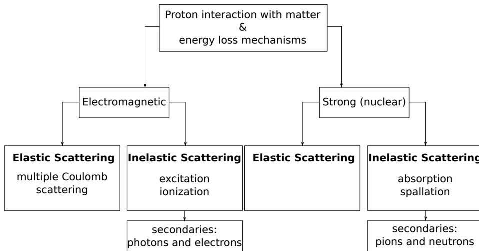
Figure 2.1: The overview of the proton interaction processes with matter and a list of some of the secondary particles produced. The processes are of statistical nature and occur with a certain probability each.
